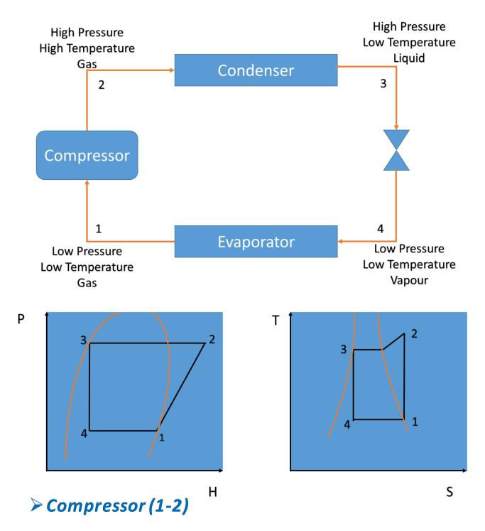
It compresses the refrigerant to high pressure. So, it gets heated.
