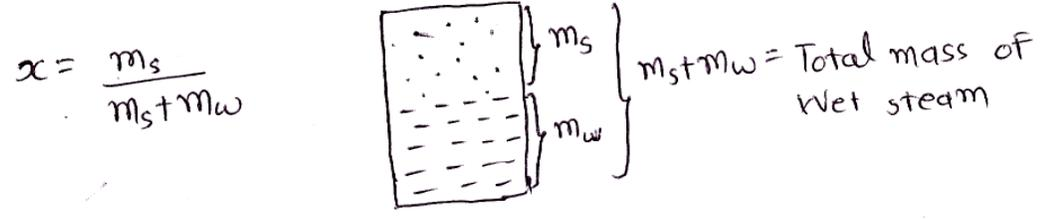
\* Wetness fraction ( $y$ ):- Ratio of mass of water in wet steam to total mass of wet steam
