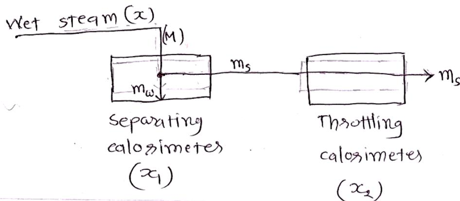
Now,  $x_1 = \frac{m_s}{m_s + m_w}$  and  $x_2 = \frac{h_{g2} + c_{ps}(T_{sup} - T_{sat}) - h_{s1}}{h_{fg1}}$
