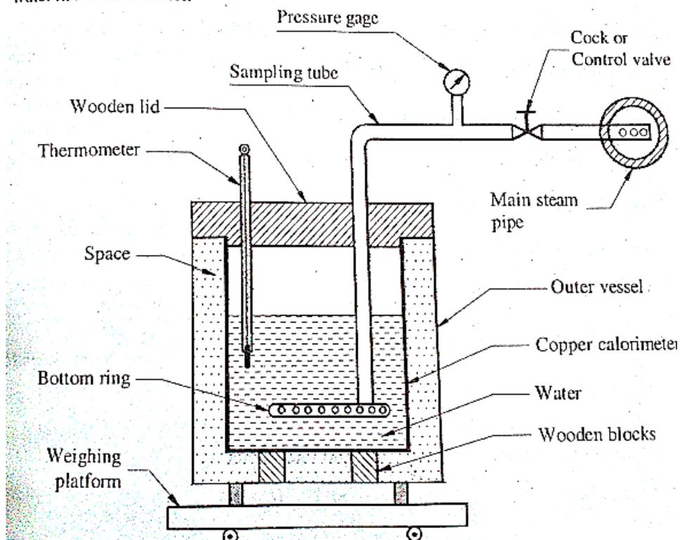
Heat lost by steam = Heat gain by water & calorimeter
